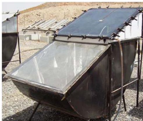
Fig. 11: Inverted absorber solar still [36].
