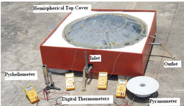
Fig. 9: Pictorial view of hemispherical solar still [33].
