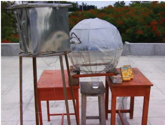
Fig. 8: Pictorial view of pyramid solar still [33].
